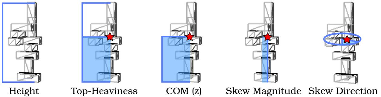
Figure 3.2: **Geometric prediction heuristics.** *Height* is the difference between the base of the lowest block and the top of the highest block along the vertical ( $z$ ) dimension. *Top-heaviness* is the ratio of the  $z$ -coordinate of the center of mass to the height of the tower. *COM (z)* is the  $z$ -coordinate of the center of mass. *Skew magnitude* and *skew direction* are (respectively) the radius and angle in cylindrical coordinates of the tower’s center of mass.
