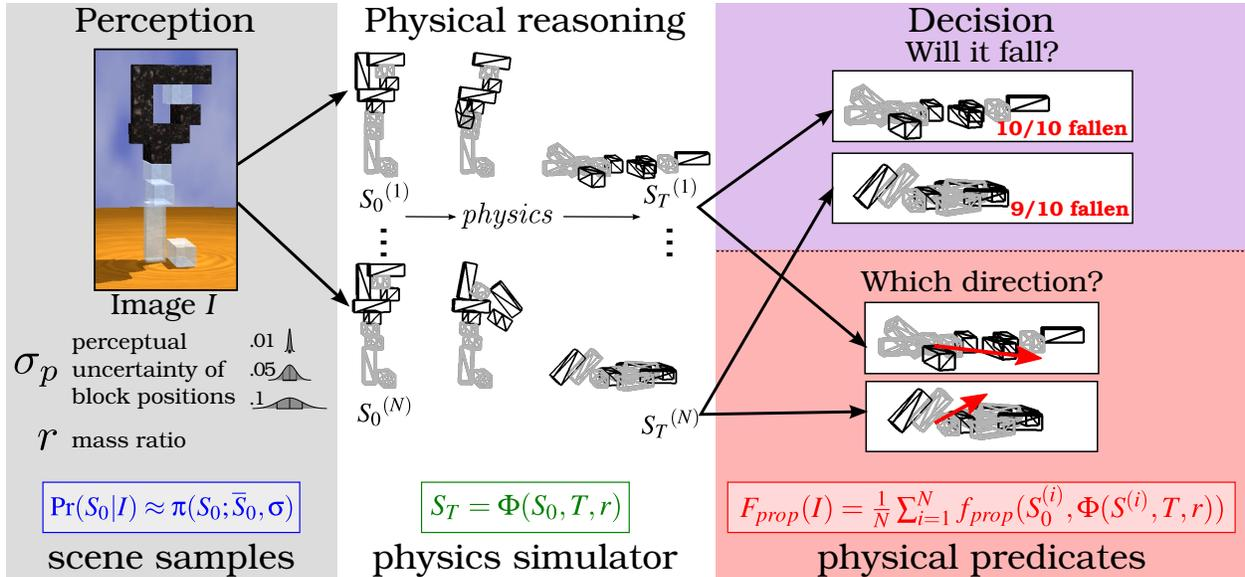
Figure 3.1: **Prediction model schematic.** Our model has 3 components, perception, physical reasoning, and decision. During perception, an uncertain belief about the tower is inferred from an image. During physical reasoning, tower samples are drawn from this belief distribution, and a physical simulation is applied to each. To make decisions about physical properties, the simulation outcomes are evaluated and averaged.
